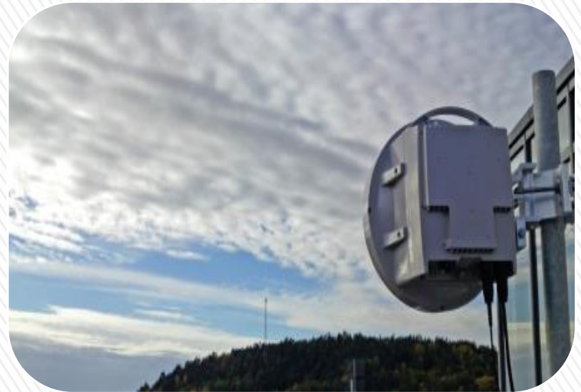
PANORAMA Point to point Communications using millimeter wave signals
